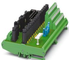
16-channel analog module with a screw connection and a fuse for each signal path (5 x 20 mm) with failure indication (LED). The voltage supply and the 40-pos. system connection are designed redundantly. Suitable for the Yokogawa AAI141 and AAI143 cards.
