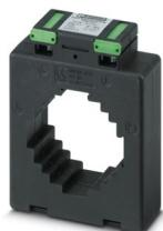
Window-type current transformer, 1,600 A AC primary current; 5 A AC secondary current; accuracy class 1; 15 VA rated power
