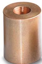
A copper sleeve for establishing a conductive connection for the horizontal installation of PACT current transformers. The size of the copper sleeve depends on the diameter of the inner hole of the current transformer. Ø 28/12 mm for PACT MCR-V2-3015-60-...
