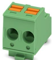
PCB connector, nominal cross section: 1.5 mm<sup>2</sup>, color: green, nominal current: 10 A, rated voltage (III/2): 400 V, contact surface: Sn, contact connection type: Socket, number of potentials: 2, number of rows: 1, number of positions: 2, number of connections: 2, product range: PTS 1,5/.-PH CLIP, pitch: 5 mm, connection method: Push-in spring connection, conductor/PCB connection direction: 0 °, plug-in system: COMBICON PST 1,3, locking: without, type of packaging: packed in cardboard
