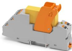
Relay module with Push-in connection, consisting of: relay base with status LED, freewheeling diode, and retaining bracket, safety relay with force-guided contacts in accordance with DIN EN 61810-3, contact switching type: 5 N/O contacts and 1 N/C contact, input voltage: 24 V DC
