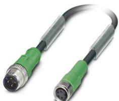
Sensor/actuator cable, 4-position, PUR halogen-free, black-gray RAL 7021, Plug straight M12, coding: A, on Socket straight M8, coding: A, cable length: 1.5 m
