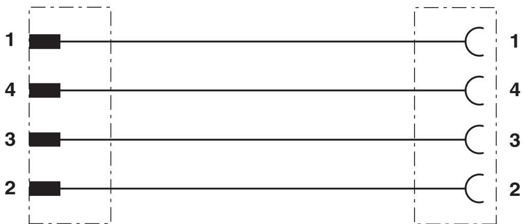
Contact assignment of M12 plugs / M8 sockets
