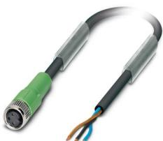
Sensor/actuator cable, 3-position, PUR halogen-free, black-gray RAL 7021, free cable end, on Socket straight M8, coding: A, cable length: 3 m
