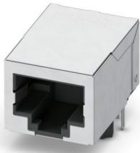
Filtered RJ45 PCB connectors, 1x1 single-port, connection direction of the connector to the PCB: 90 °, Tab down, Shielded, number of positions: 8, 1 Gbps, THT, Wave, type of packaging: Tray
