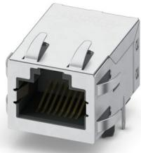
Filtered RJ45 PCB connectors, 1x1 single-port, connection direction of the connector to the PCB: 90 °, Tab up, Shielded, shield springs, number of positions: 8, 1 Gbps, THT, Wave, type of packaging: Tray
