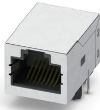
Filtered RJ45 PCB connectors, 1x1 single-port, connection direction of the connector to the PCB: 90 °, Tab up, Shielded, number of positions: 8, 1 Gbps, THT, Wave, type of packaging: Tray
