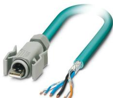
Assembled USB cable, shielded, color: RAL 5021 (water blue), PUR outer sheath, USB type A/IP67 on open cable end, length: 5 m
