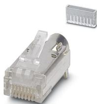
RJ45 pin insert, CAT5, 8-pos., shielded, IDC connection technology, for 27 ... 26 AWG litz wires, with strain relief
