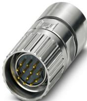
M23, Cable connector, series: M23 PRO, straight, shielded: yes, Screw locking mechanism, No. of pos.: 12, Direction of rotation: Standard, contact connection type: Pin, Crimp connection, cable diameter range: 6 mm ... 10 mm, coding: N, Item is lead-free in accordance with RoHS II without Exemption 6c (Pb < 0.1 %)
