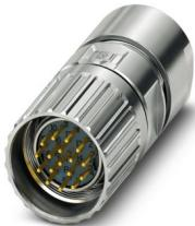
M23, Cable connector, series: M23 PRO, straight, shielded: yes, Screw locking mechanism, No. of pos.: 17, Direction of rotation: Standard, contact connection type: Pin, Crimp connection, cable diameter range: 9 mm ... 15 mm, coding: N, Item is lead-free in accordance with RoHS II without Exemption 6c (Pb < 0.1 %)
