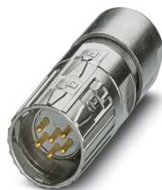
M23, Cable connector, series: M23 PRO, straight, shielded: yes, ONECLICK fast locking system, No. of pos.: 6, Direction of rotation: Standard, contact connection type: Pin, Crimp connection, cable diameter range: 9 mm ... 15 mm, coding: N, Item is lead-free in accordance with RoHS II without Exemption 6c (Pb < 0.1 %)
