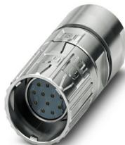
M23, Cable connector, series: M23 PRO, straight, shielded: yes, ONECLICK fast locking system, No. of pos.: 12, Direction of rotation: Standard, contact connection type: Socket, Crimp connection, cable diameter range: 6 mm ... 10 mm, coding: N, Item is lead-free in accordance with RoHS II without Exemption 6c (Pb < 0.1 %)
