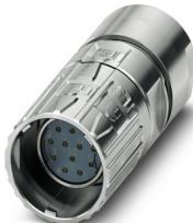
M23, Cable connector, series: M23 PRO, straight, shielded: yes, ONECLICK fast locking system, No. of pos.: 12, Direction of rotation: Standard, contact connection type: Socket, Crimp connection, cable diameter range: 9 mm ... 15 mm, coding: N, Item is lead-free in accordance with RoHS II without Exemption 6c (Pb < 0.1 %)
