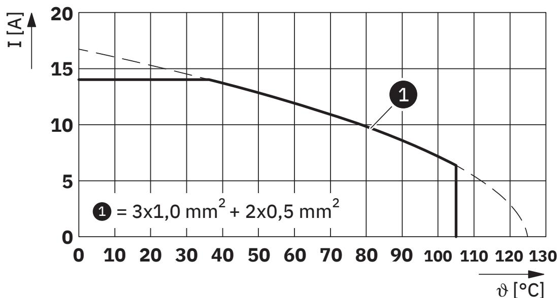
$I$  = current strength,  $\vartheta$  = ambient temperature,  $3 \times 14 \text{ A} + 2 \times 2 \text{ A}$  constant
