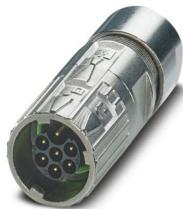
M17, Cable connector, series: M17 PRO, straight, shielded: yes, ONECLICK fast locking system, No. of pos.: 6+PE, contact connection type: Pin, Crimp connection, cable diameter range: 5.5 mm ... 9.5 mm, Item is lead-free in accordance with RoHS II without Exemption 6c (Pb < 0.1 %)
