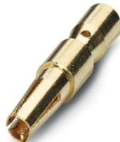
Crimp contact, Socket, turned, contact diameter: 1.5 mm, connection cross section: 0.5 mm<sup>2</sup> ... 1 mm<sup>2</sup>, contact material: CuZn, Alternative product in accordance with RoHS II without Exemption 6c (Pb < 0.1 %) item no.: 1244969
