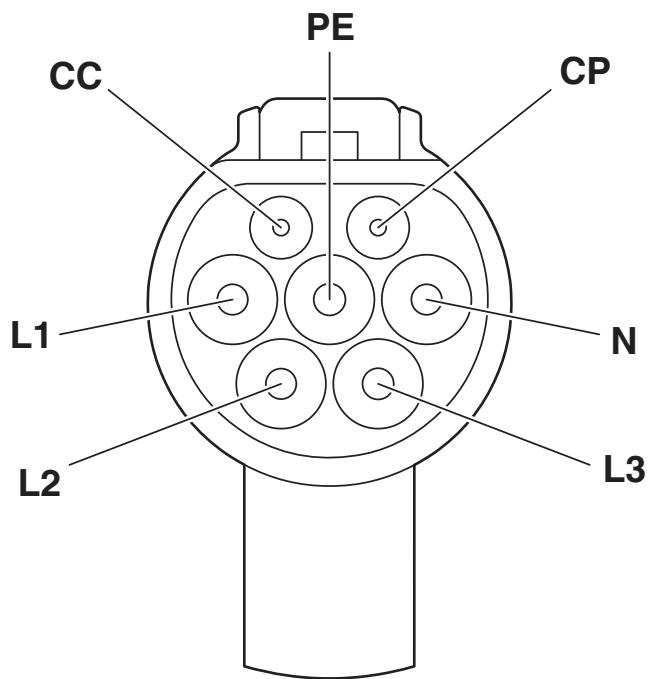
Pin assignment of the Vehicle Connector
