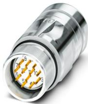
M23, Coupler connector, series: CA, straight, shielded: yes, for standard and SPEEDCON interlock, No. of pos.: 12, Direction of rotation: Standard, contact connection type: Pin, Solder cup, cable diameter range: 10 mm ... 14.5 mm, coding: N. This product is in the process of being discontinued. This product must no longer be considered for new projects. Please contact your sales representative for alternatives.
