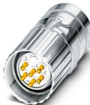
M23, Cable connector, series: CA, straight, shielded: yes, Screw locking mechanism, No. of pos.: 6, Direction of rotation: Standard, contact connection type: Pin, Solder connection, cable diameter range: 4 mm ... 6 mm, coding: N. This product is in the process of being discontinued. This product must no longer be considered for new projects. Please contact your sales representative for alternatives.
