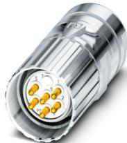
M23, Cable connector, series: CA, straight, shielded: yes, Screw locking mechanism, No. of pos.: 8+1, Direction of rotation: Standard, contact connection type: Pin, Crimp connection, cable diameter range: 6 mm ... 10 mm, coding: N. This product is in the process of being discontinued. This product must no longer be considered for new projects. Please contact your sales representative for alternatives.
