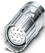
M23, Cable connector, series: CA, straight, shielded: yes, Screw locking mechanism, No. of pos.: 12, Direction of rotation: Standard, contact connection type: Socket, Solder connection, cable diameter range: 6 mm ... 10 mm, coding: N. This product is in the process of being discontinued. This product must no longer be considered for new projects. Please contact your sales representative for alternatives.
