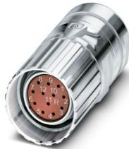
M23, Cable connector, series: CA, straight, shielded: yes, Screw locking mechanism, No. of pos.: 12, Direction of rotation: Standard, contact connection type: Socket, Crimp connection, cable diameter range: 3 mm ... 14.5 mm, coding: N. This product is in the process of being discontinued. This product must no longer be considered for new projects. Please contact your sales representative for alternatives.
