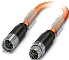
Connector in molded plastic on both sides, series: KST, M17-Socket, Straight, plastic molded, number of positions: 5+PE, type of locking: Screw locking mechanism, on M17-Pin, Straight, plastic molded, number of positions: 5+PE, cable length: 2 m, shielded: yes, this item is expected to be lead-free from Q1 2027 in accordance with RoHS II without exception 6c (Pb < 0.1%), a lead-free alternative is possible on request in advance
