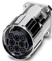
Device connector front mounting with knurled nut, straight, Screw locking mechanism, M40, number of positions: 2+3+PE, contact connection type: Socket, Axial O-ring, shielded: yes, flange dimensions: 40 mm x 40 mm, cable diameter range: 0 mm ... 0 mm, number of positions: 6, connection method: Crimp connection, series: SM, this item is expected to be lead-free from Q3 2026 in accordance with RoHS II without exception 6c (Pb < 0.1%), a lead-free alternative is possible on request in advance
