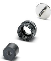
Cable clamp type cage and shield adapter, shielded: yes, litz wire bundle diameter: 4.1 mm, cable diameter range: 6.5 mm ... 7.5 mm, series: NC, RC
