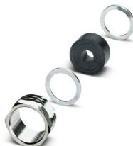
Cable gland, material for screw connection: Brass, nickel-plated, external cable diameter 6 mm .. . 10 mm, shielding: no, connecting thread: Pg9, series: RC, this item is expected to be lead-free from Q4 2025 in accordance with RoHS II without exception 6c (Pb < 0.1%), a lead-free alternative is possible on request in advance
