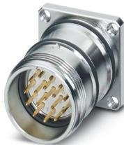
M23, Device connector front mounting, series: RC, straight, shielded: yes, Screw locking mechanism, No. of pos.: 7, Direction of rotation: Standard, contact connection type: Pin, Crimp connection, Radial O-ring, Panel thickness min.: 3 mm, Panel thickness max.: 10.5 mm, coding: N. This product is in the process of being discontinued. This product must no longer be considered for new projects. Please contact your sales representative for alternatives.
