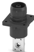
Connector, Range of articles: BPC 250, color: black, number of positions: 1, rated voltage: 1500 V DC, rated current: 250 A, Connection method: Thread connection, min. cable diameter: 9.7 mm, max. cable diameter: 17.8 mm
