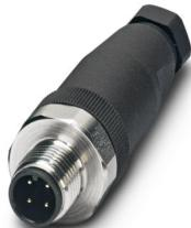
Connector, Universal, 4-position, Plug straight M12, coding: A, Screw connection, knurl material: Stainless steel 1.4404, cable gland Pg7, external cable diameter 4 mm ... 6 mm
