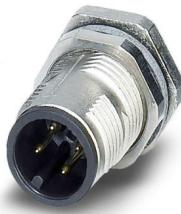
Device connector rear mounting, 4-position, Pin, straight, M12-SPEEDCON, A-coding, Wave soldering, this item is expected to be lead-free from Q2 2026 in accordance with RoHS II without exception 6c (Pb < 0.1%), a lead-free alternative is possible on request in advance
