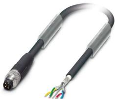
Bus system cable, INTERBUS, 4-position, PUR halogen-free, black RAL 9005, shielded, Plug straight M8, coding: A, on free cable end, cable length: 20 m
