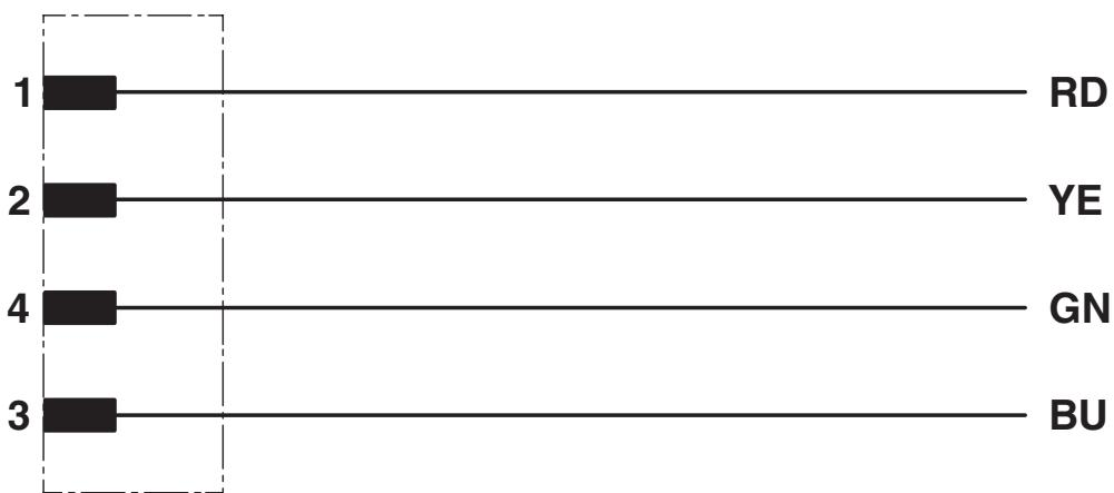
Contact assignment of the M8 plug
