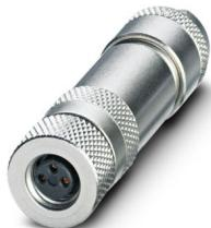
Connector, Universal, 3-position, shielded, Socket straight M8, coding: A, Screw connection, knurl material: Brass, nickel-plated, external cable diameter 3.5 mm ... 5.5 mm
