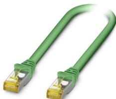
Patch cable, RJ45/IP20 straight on RJ45/IP20 straight, cable length: 12.5 m, number of positions: 8, CAT6<sub>A</sub>, connection cross section: AWG 26- 26, Ethernet, 4x2xAWG26/7; S/FTP, green
