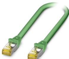
Patch cable, RJ45/IP20 straight on RJ45/IP20 straight, cable length: 7.5 m, number of positions: 8, CAT6<sub>A</sub>, connection cross section: AWG 26- 26, Ethernet, 2x2xAWG26/7, S/UTP, green
