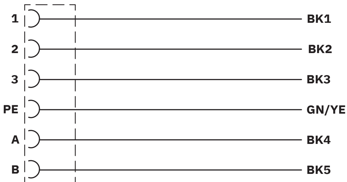
Contact assignment of the M12 socket
