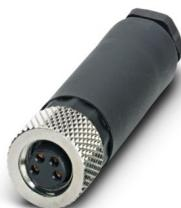
Connector, Universal, 4-position, Socket straight M8, coding: A, Screw connection, knurl material: Brass, nickel-plated, external cable diameter 3.5 mm ... 5 mm
