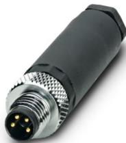
Connector, Universal, 4-position, Plug straight M8, coding: A, Screw connection, knurl material: Brass, nickel-plated, external cable diameter 3.5 mm ... 5 mm
