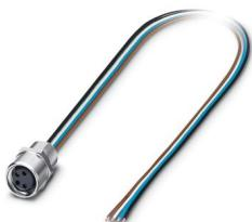
Device connector front mounting, 4-position, Socket, straight, M8, A-coding, Individual wires, cable length: 0.5 m, 0.25 mm<sup>2</sup>, PVC litz wire
