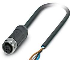
Sensor/actuator cable, 4-position, PE-X halogen-free, black-gray RAL 7021, free cable end, on Socket angled M12, coding: A, cable length: 65 m, for outdoor applications, with high-grade steel knurl
