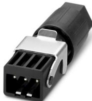
Connector, connection method: IDC connection, number of positions: 3+PE, 0.5 mm<sup>2</sup> ... 1.5 mm<sup>2</sup>, 400 V, 16 A AC/DC, black, with one QUICKON nut, external cable diameter: 7 mm ... 13 mm, Connectors for the motor connection of Venetian blinds, blinds, roller shutters, and awnings
