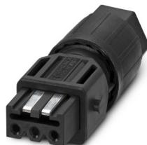
Connector, connection method: IDC connection, number of positions: 3+PE, 0.5 mm<sup>2</sup> ... 1.5 mm<sup>2</sup>, 400 V, 16 A AC/DC, black, with one QUICKON nut, external cable diameter: 7 mm ... 13 mm, Connectors for the motor connection of Venetian blinds, blinds, roller shutters, and awnings
