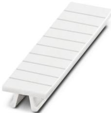
Zack marker strip, Strip, white, unmarked, can be labeled with: PLOTMARK, CMS-P1-PLOTTER, mounting type: latching, for terminal block width: 4.2 mm, Number of individual labels: 10, text field height: 10.5 mm, text field width: 4.2 mm
