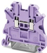
Feed-through terminal block, nom. voltage: 1000 V, nominal current: 17.5 A, number of connections: 2, connection method: Screw connection, Rated cross section: 1.5 mm<sup>2</sup>, cross section: 0.14 mm<sup>2</sup> - 1.5 mm<sup>2</sup>, mounting type: NS 35/7,5, NS 35/15, color: violet
