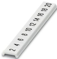
Zack Marker strip, flat, Strip, white, labeled, printed horizontally: consecutive even numbers 2 ... 20, 22 ... 40, etc. up to 82 ... 100, mounting type: latching, for terminal block width: 4 mm, Number of individual labels: 10, text field height: 5.15 mm, text field width: 4.15 mm
