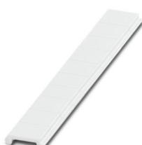
Zack Marker strip, flat, can be ordered: Strip, white, labeled according to customer specifications, mounting type: snap into flat marker groove, for terminal block width: 4.2 mm, Number of individual labels: 10, text field height: 5.2 mm, text field width: 4.2 mm
