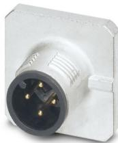
Device connector front mounting, Universal, 4-position, Pin, straight, M12-SPEEDCON, A-coding, Wave soldering, 0.34 mm<sup>2</sup>, this item is expected to be lead-free from Q4 2025 in accordance with RoHS II without exception 6c (Pb < 0.1%), a lead-free alternative is possible on request in advance
