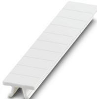
Zack marker strip, Strip, white, unmarked, can be labeled with: PLOTMARK, CMS-P1-PLOTTER, mounting type: latching, for terminal block width: 5.2 mm, Number of individual labels: 10, text field height: 10.5 mm, text field width: 5.1 mm
