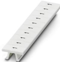
Zack marker strip, Strip, white, labeled, can be labeled with: CMS-P1-PLOTTER, printed horizontally: Identical numbers 1 or 2, etc. up to 100, mounting type: latching, for terminal block width: 5.2 mm, Number of individual labels: 10, text field height: 10.5 mm, text field width: 5.15 mm
