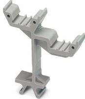
Marker carriers, snaps into ST 2,5 spring-cage terminal blocks, can be marked with UC-TM 5, UC-TMF 5, UCT-TM 5, UCT-TMF 5, ZB 5, or ZBF 5, gray, unmarked, mounting type: latching, text field height: 10.5 mm, text field width: 5 mm
