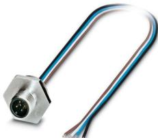
Device connector front mounting, 5-position, Pin, straight, M12-Standard, A-coding, on free cable end, Individual wires, cable length: 0.5 m, 0.34 mm<sup>2</sup>, TPE litz wire, potted
