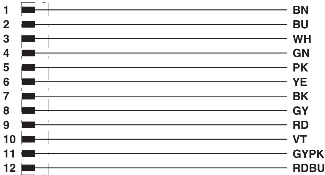
Contact assignment of the M12 plugs
