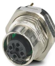
Device connector rear mounting, 4-position, Socket, straight, M12-SPEEDCON, D-coding, Wave soldering, this item is expected to be lead-free from Q1 2026 in accordance with RoHS II without exception 6c (Pb < 0.1%), a lead-free alternative is possible on request in advance
